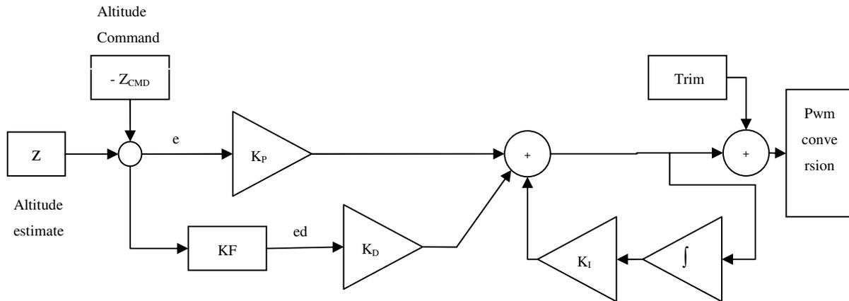
Figure 4. Schematic of Altitude Hold Control System
