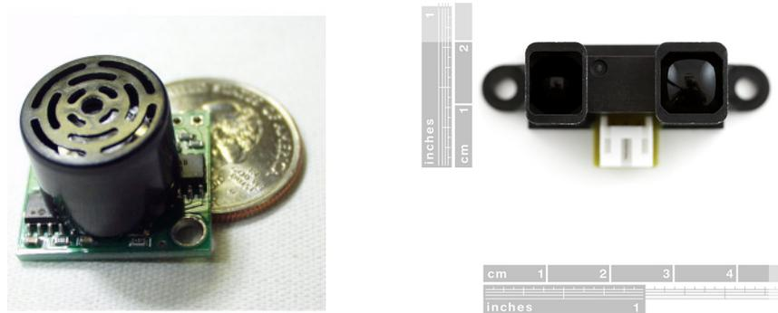
*Figure 5. Primary range sensors are the MaxBotix® LV-MaxSonar® (on the left), and the SHARP GP2Y0A02YK0F infrared range sensor (on the right). Photos courtesy SparkFun Electronics: [www.sparkfun.com](http://www.sparkfun.com).*
