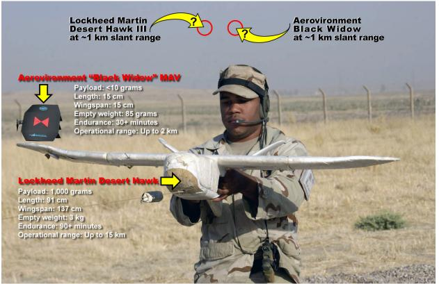
*Figure 1. Simulated comparison of the Desert Hawk mini drone and the Aerovironment Black Widow MAV flying at 500 meters above ground level at a range of 1 km (1.118 km slant range).*
