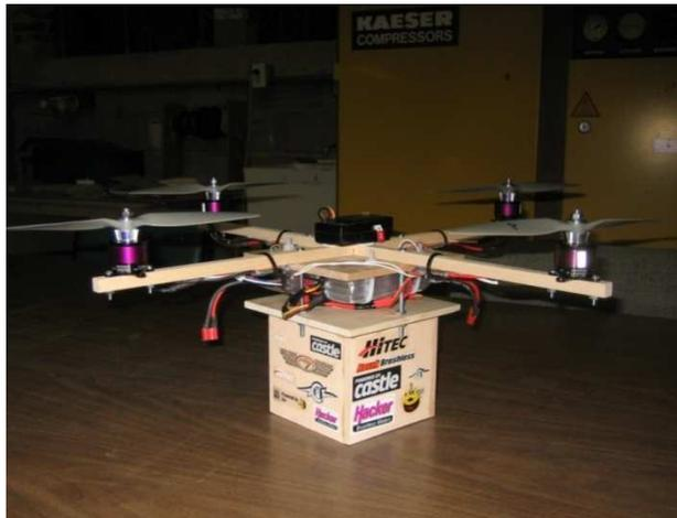
*Figure 6. Photograph of the first vehicle prototype.*
