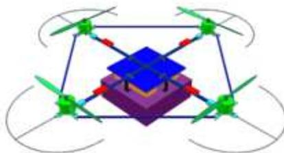
*Figure 7. This is a diagram of the aluminum safety bumpers on the quad-rotor*
