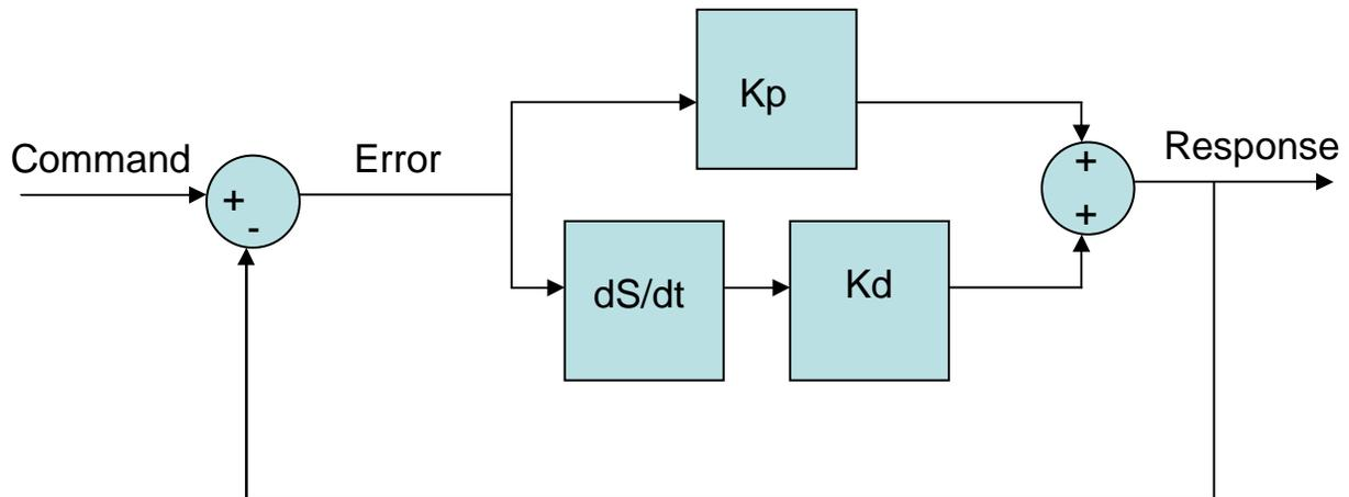
Figure 2. The block diagram representation of a PD control loop. This loop is used to stabilize the vehicle.
