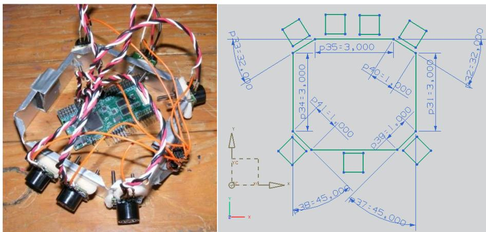
Figure 4. A picture and diagram of the test sensor bracket. The dimensions are shown (right) and the current state is shown (left)
