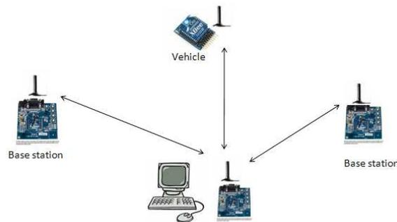
*Figure 5. This shows 'point to multipoint' used for data communication systems. It will be necessary to add another point that will be with the judges for the JAUS protocol.*
