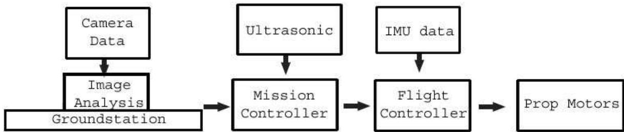
Figure 1. This plot shows the overall system architecture
