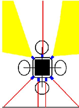
Figure 3. The red lines indicate the narrow range sensors, and the yellow areas indicate the wide range sensors. The black line at the bottom is the wall.
