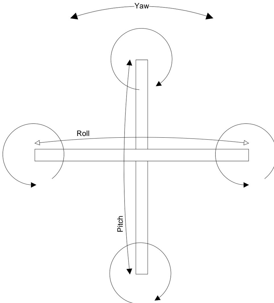
Figure 2. Aerial Vehicle Concept Diagram
