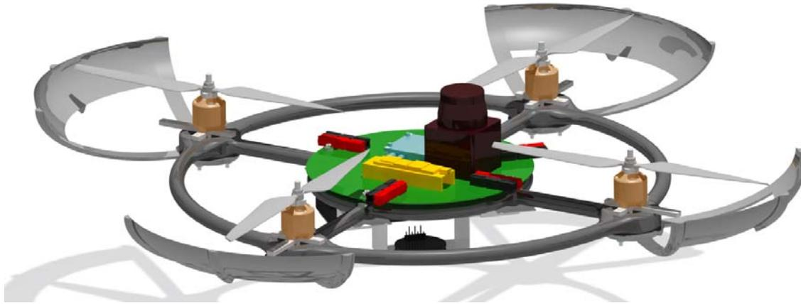
Figure 2 - MAAVerick Structure and Electronics
