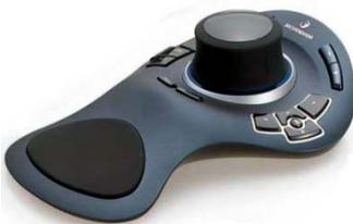
**Figure 5 - Space Explorer by 3DConnexion used to control the vehicle remotely**
