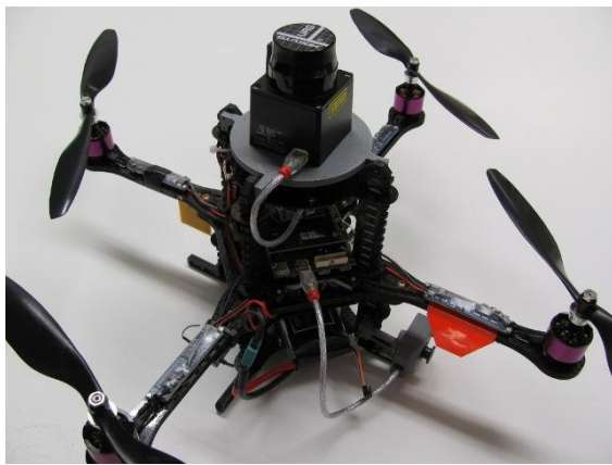
Figure 2: The Asctec Pelican quadrotor and the propeller action.
