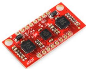
Figure 3. Razor 6-DOF IMU
