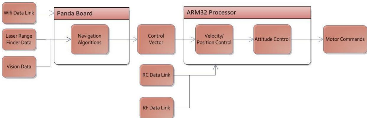
*Figure 3: Control System Architecture*
