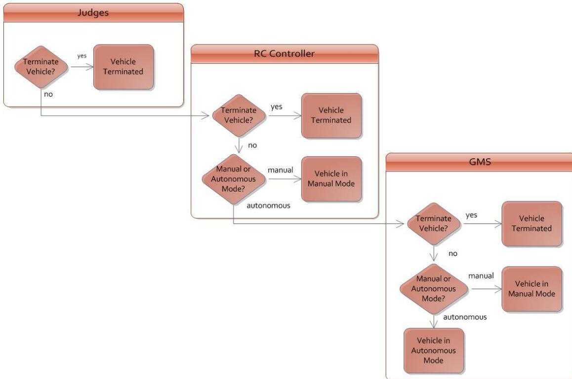
*Figure 4: Man/Machine Interface Command Hierarchy*
