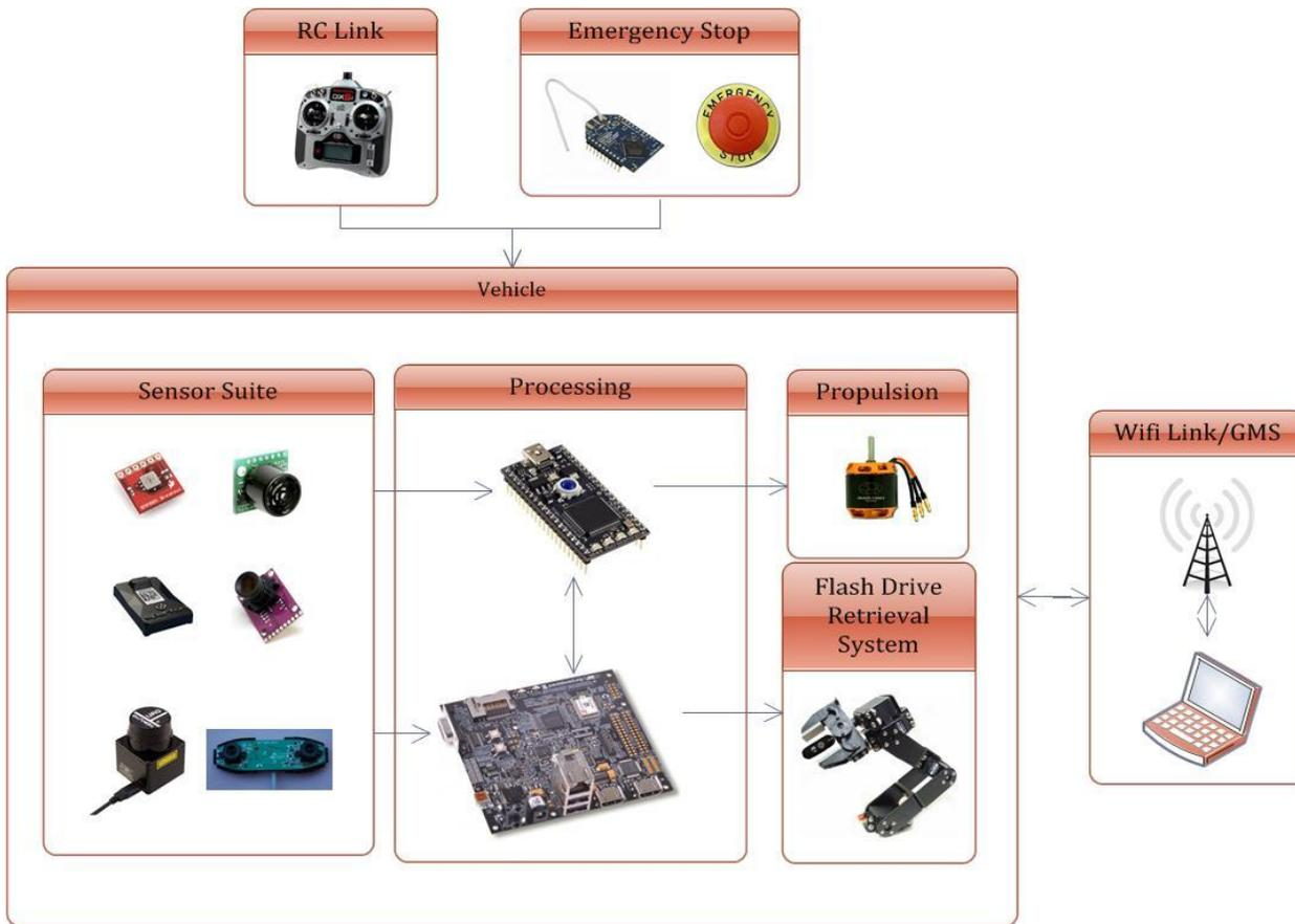
*Figure 1: ERAU Raven System Architecture*
