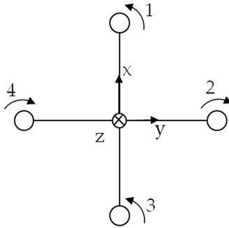
Figure 5. Quadrotor's body axis and direction of motor rotation
