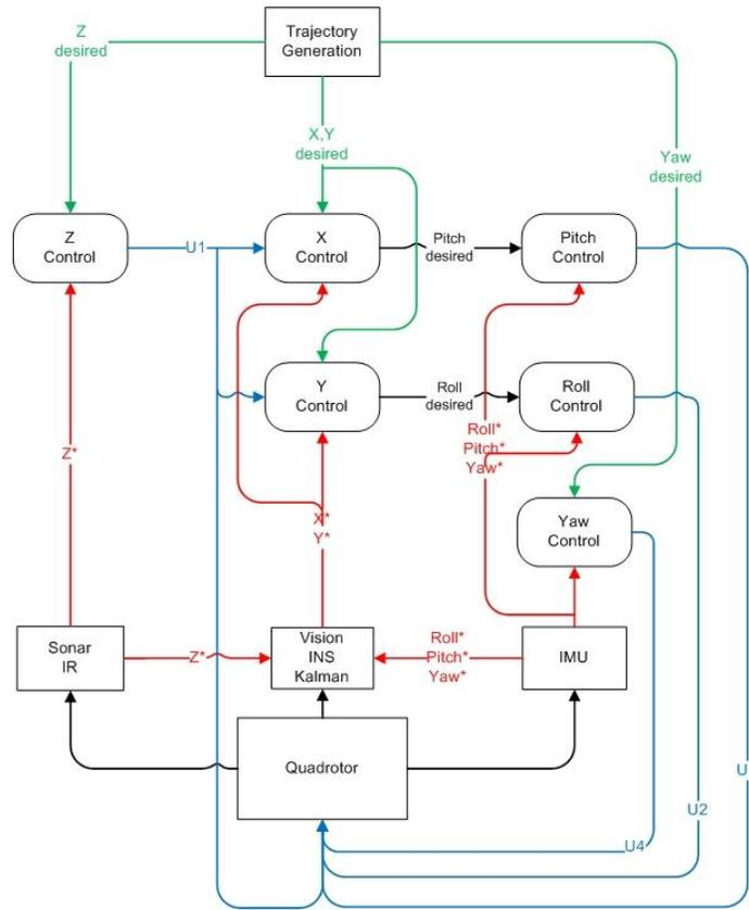
Figure 6. Nonlinear control architecture
