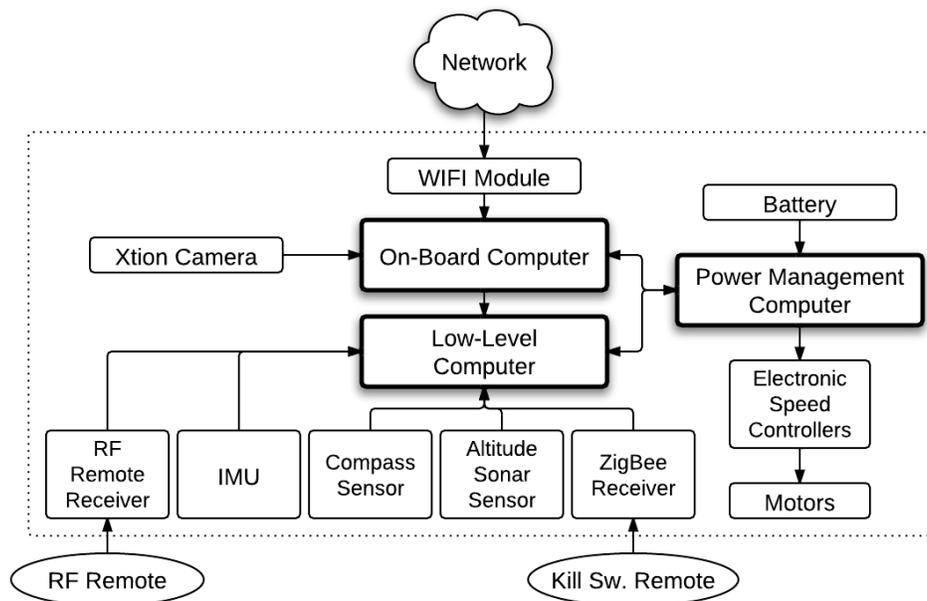
Figure 1. Hardware architecture
