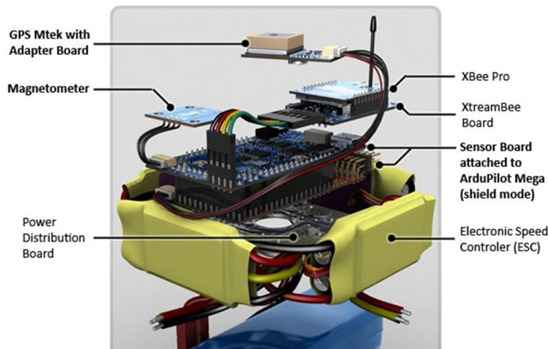
*Fig.4 Auto-Pilot System Layout*
