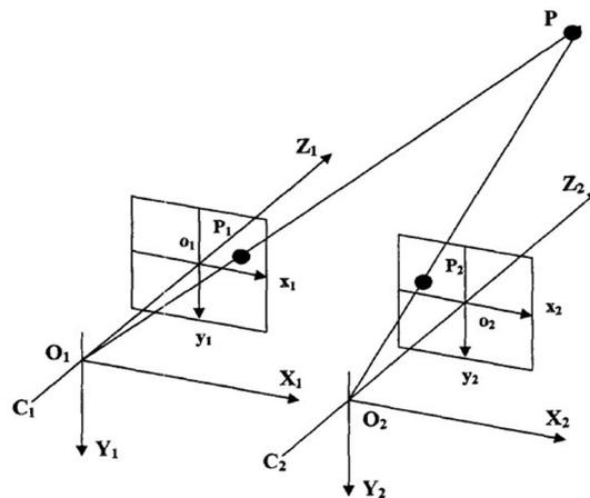
*Fig.3 Binocular vision system calibration*
