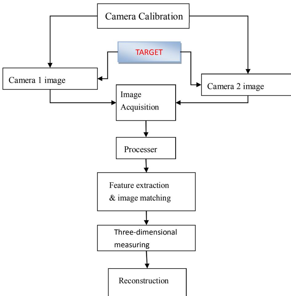
Fig.2 Camera system Module
