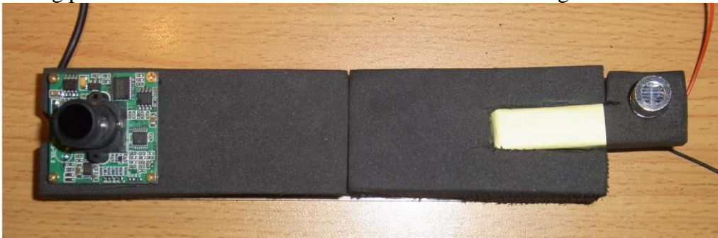
Figure 9. Self-made Laser Range Finder
