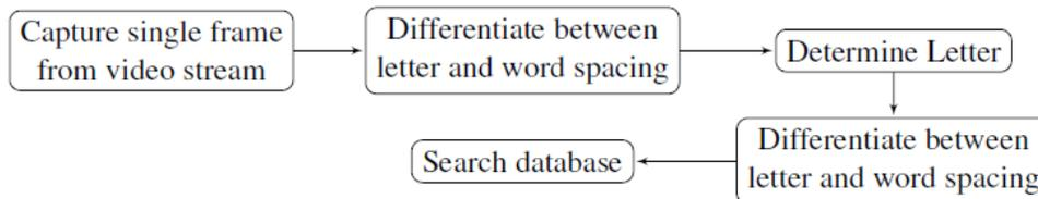
Figure 5: Flowchart showing algorithm to detect and recognize signs.
