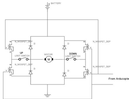
Figure 8: H-Bridge circuit drawing.
