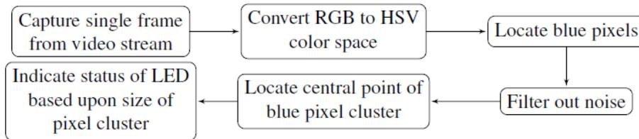
Figure 4: Flowchart Showing Algorithm to Detect Blue LED
