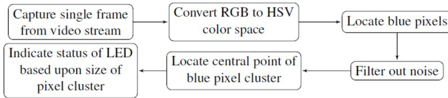
Figure 4: Flowchart Showing Algorithm to Detect Blue LED
