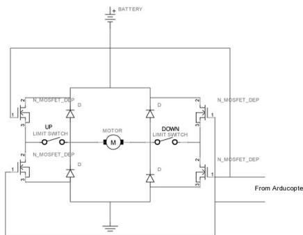
Figure 8: H-Bridge circuit drawing.
