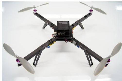
*Figure 3: Typical quad-rotor helicopter.*
