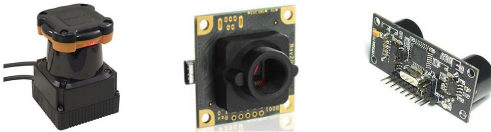
(a) Hokuyo Laser Range Finder (b) Vision light camera (c) Ultrasonic altimeter
