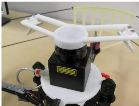
*Figure 5: LIDAR mirror mount for height estimation*
