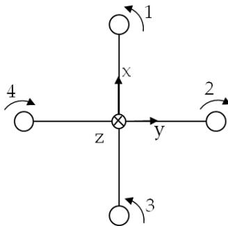
*Figure 4. Quadrotor's body axis and direction of motor rotation*
