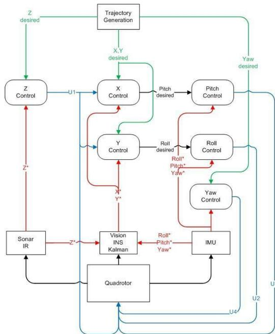
Figure 5. Nonlinear control architecture
