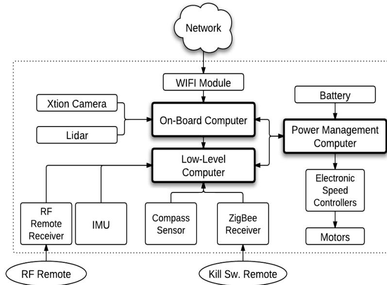
Figure 1. Hardware architecture
