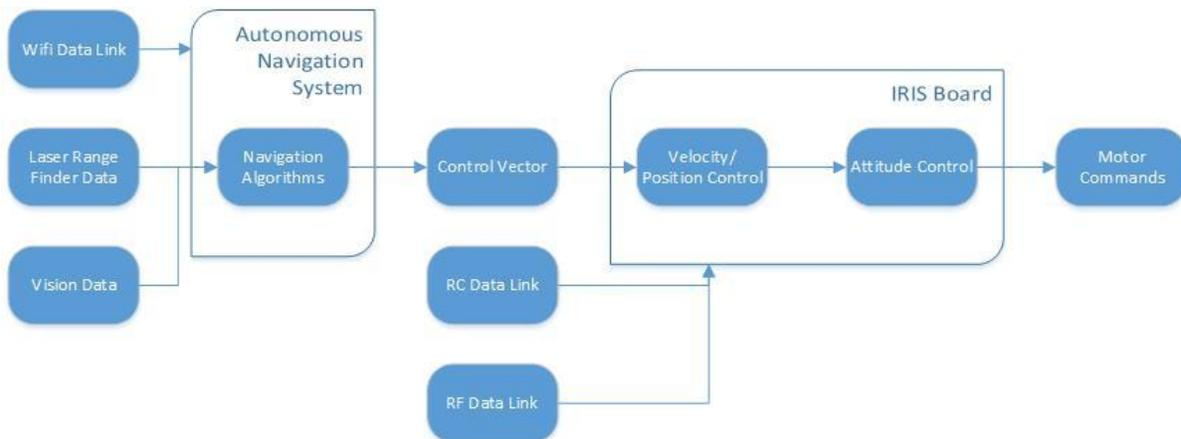
*Figure 4: Control System Architecture*
