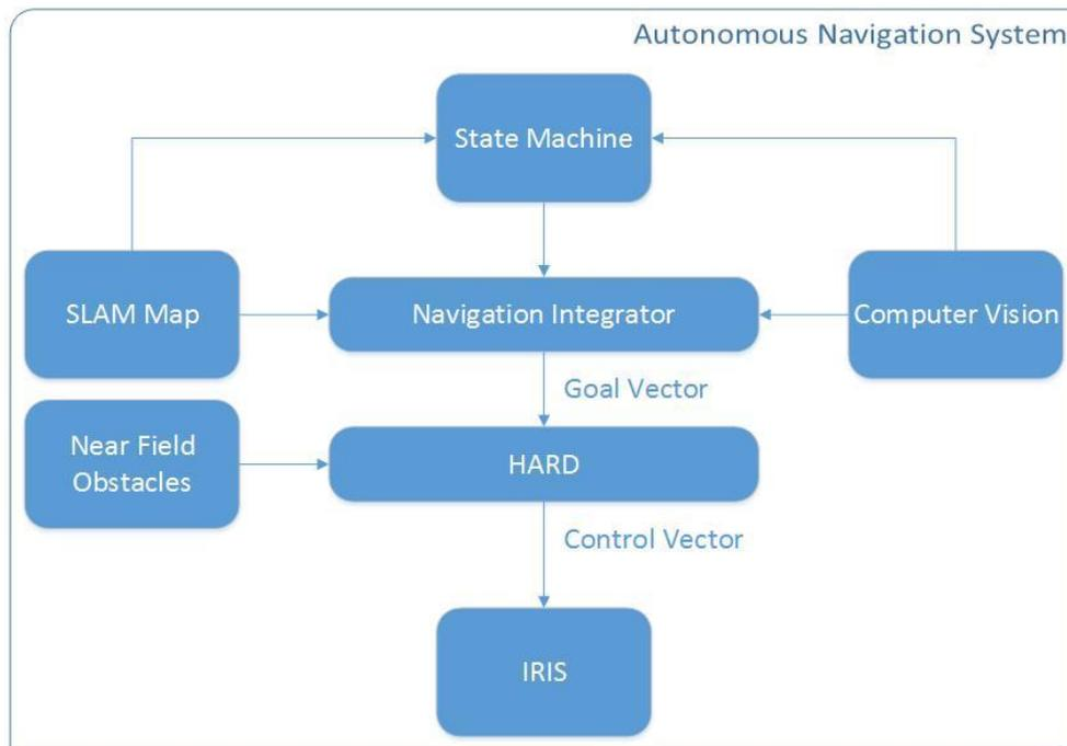
Figure 3: Autonomous Navigation System
