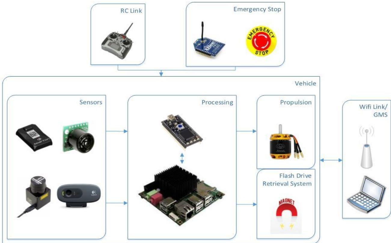
*Figure 1: ERAU Raven II System Architecture*
