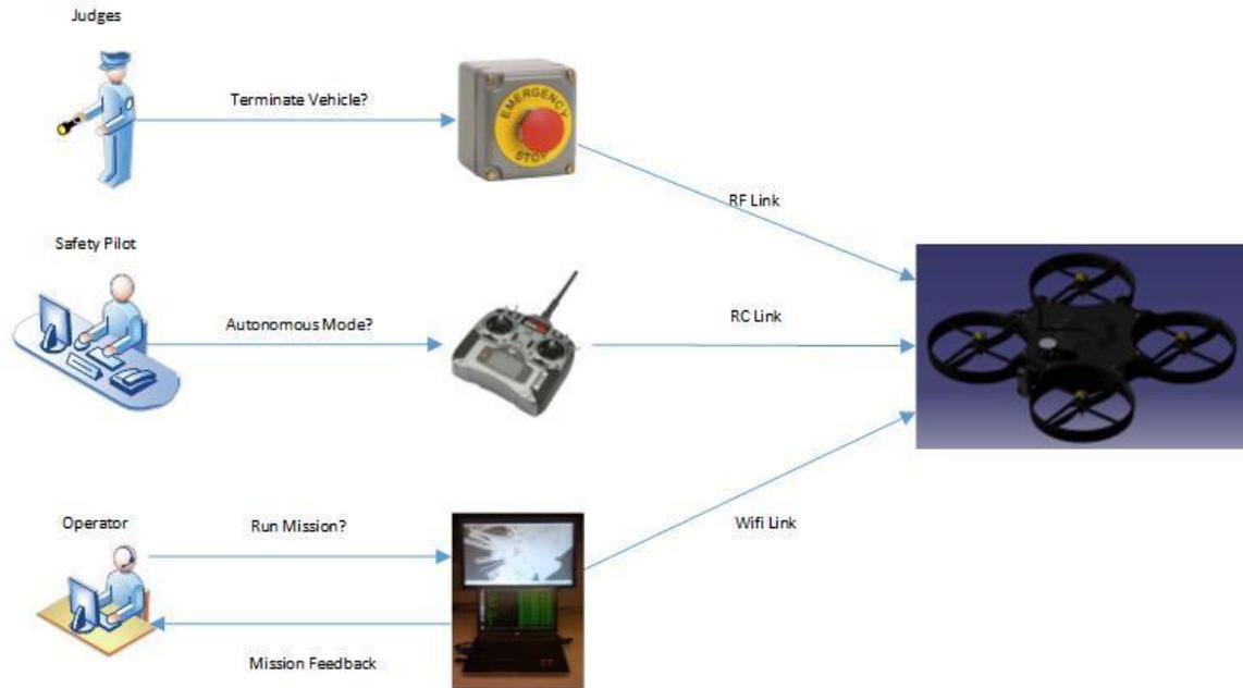
*Figure 5: Man/Machine Interface Hierarchy*
