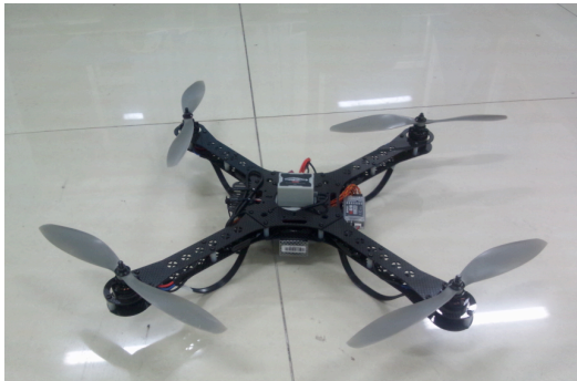
Figure 2:quadrotor and the propeller action
