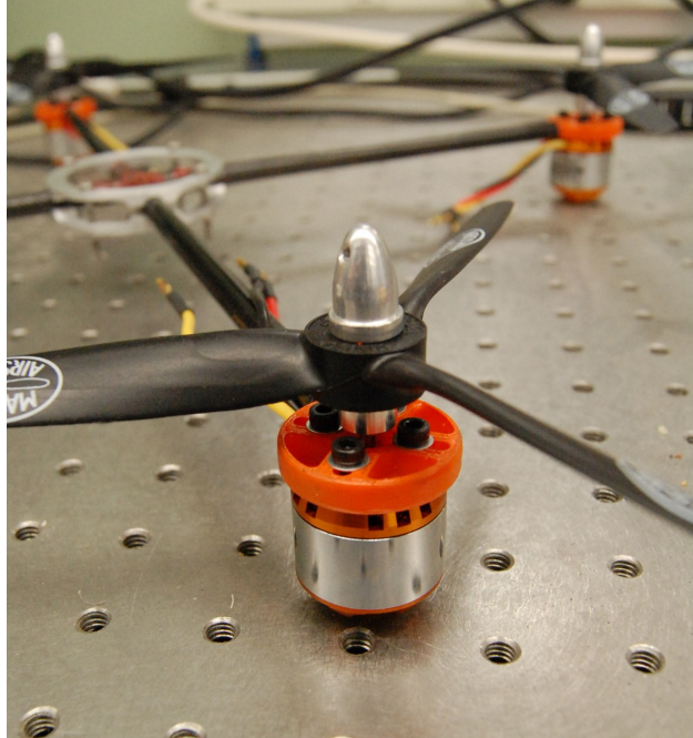
Figure 3: Final motor mount configuration. Having the two rotating masses on either side of the mount reduces vibration.
