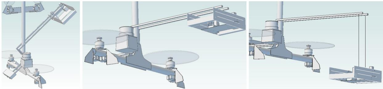
*Figure 7. Positions of retriever on vehicle. From left, stowed during flight, deployed over flash drive, lowered onto flash drive.*
