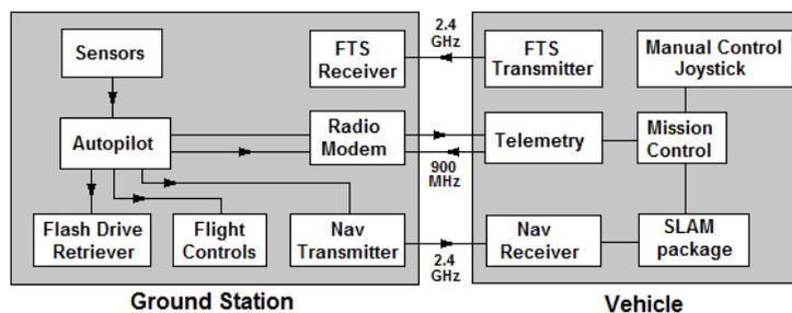
Figure 1. Overall system architecture.
