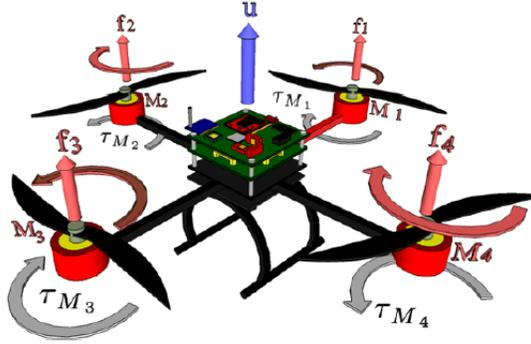
Figure 2 Basic structure of the quad-rotor [5].
