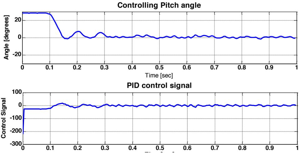
Figure 8 Tuning Pitch control loop.
