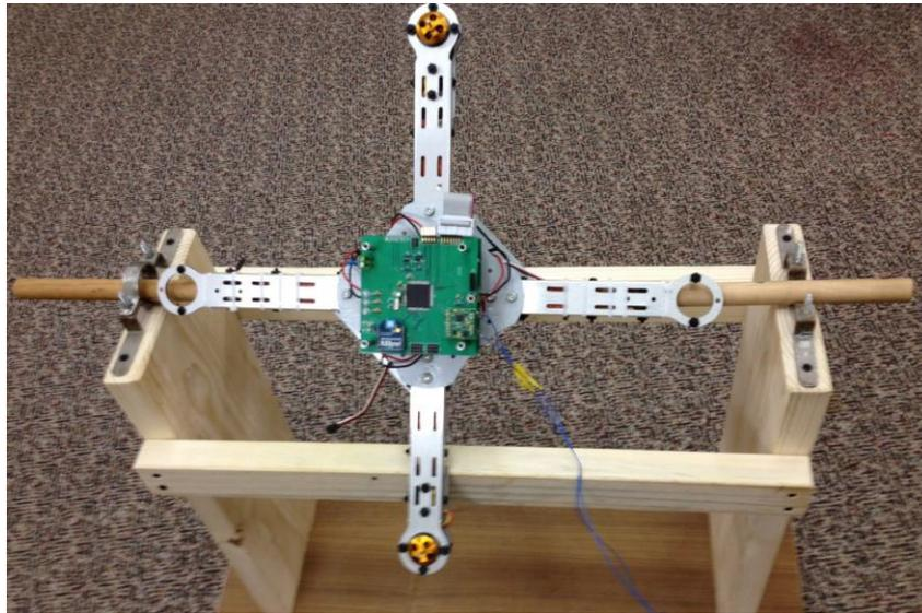
Figure 7 Testing bench for Roll and Pitch angles.
