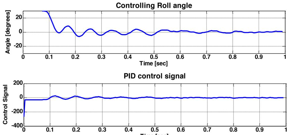
Figure 9 Tuning Roll PID controller.
