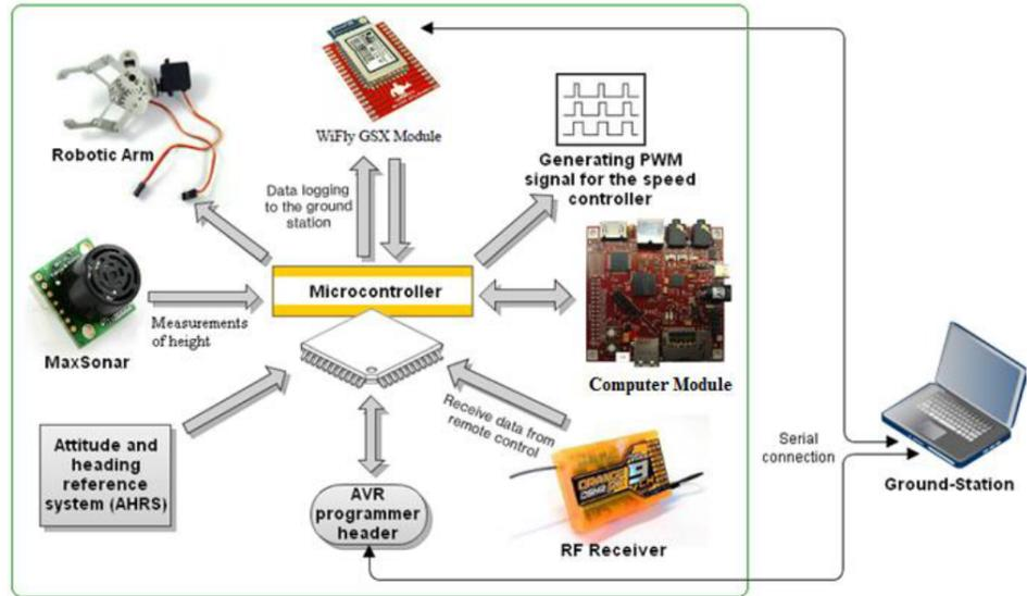
Figure 3: The Overall main Control System Structure.
