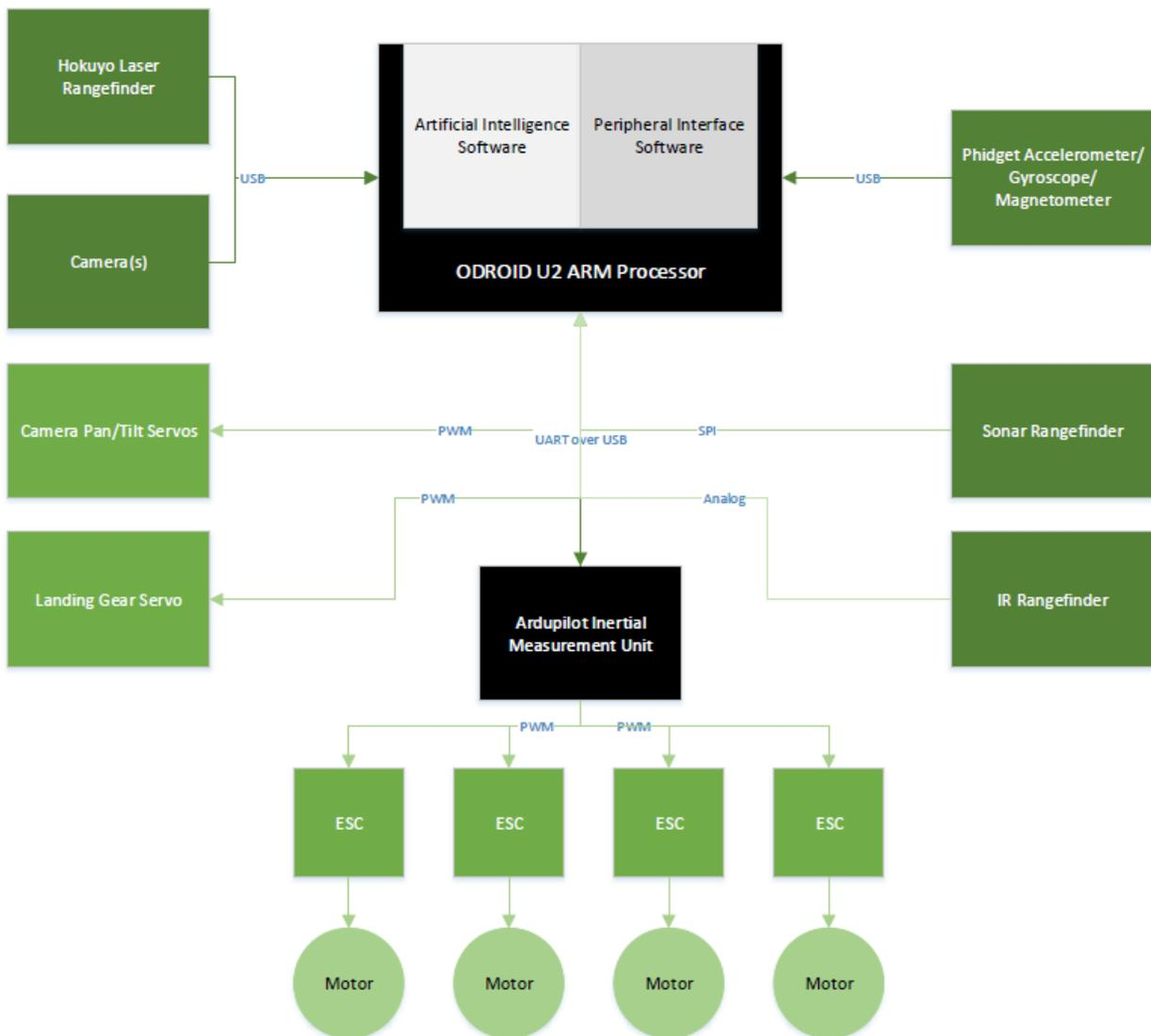
Figure 1. Control System Architecture.
