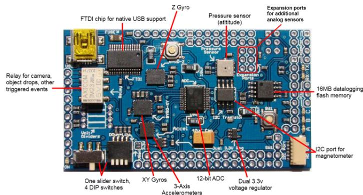
*Figure 2. ArduPilot Mega 2 Hardware Diagram.<sup>1</sup>*
