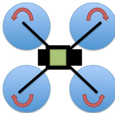
*Figure 1, Motor Configuration of the Vehicle*
