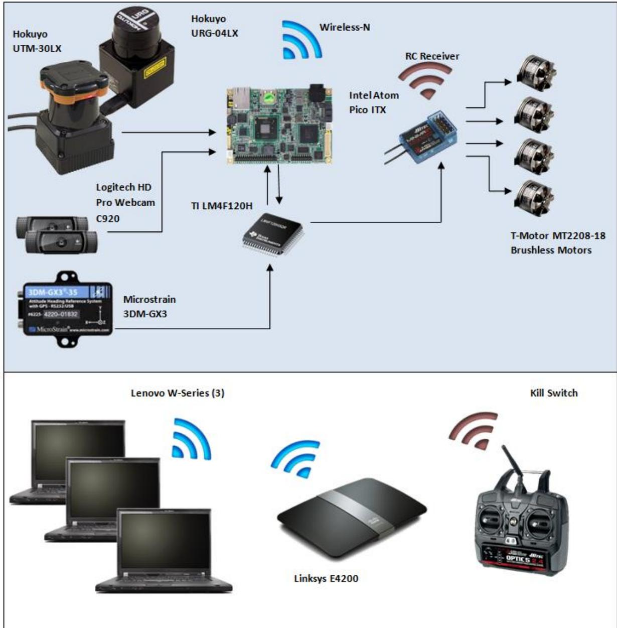
Figure 2: MAAV System Architecture
