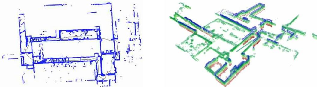
Figure 3: (left) 2D map generated with only a horizontal laser, (right) 3D map generated with both vertical and horizontal lasers
