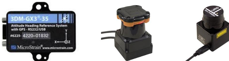
*Figure 5: The Microstrain 3DM-GX3-25 (left), Hokuyo UTM-30LX Laser Rangefinder (Center) and Hokuyo URG-04LG-UG01 Laser Rangefinder (right).*
