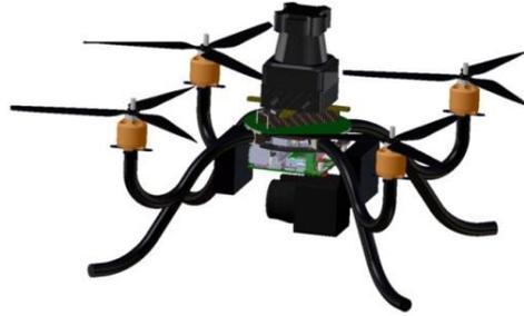
*Figure 7: A model in CATIA V5. This was used for full vehicle fabrication and assembly*
