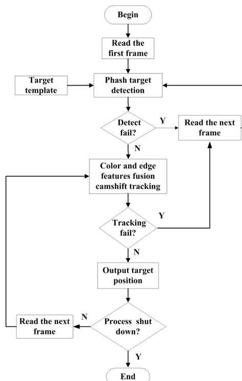
Fig2.6 Ground target tracking algorithm
