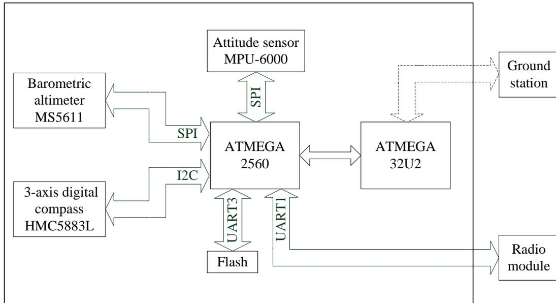
Figure3. Interface diagram of APM
