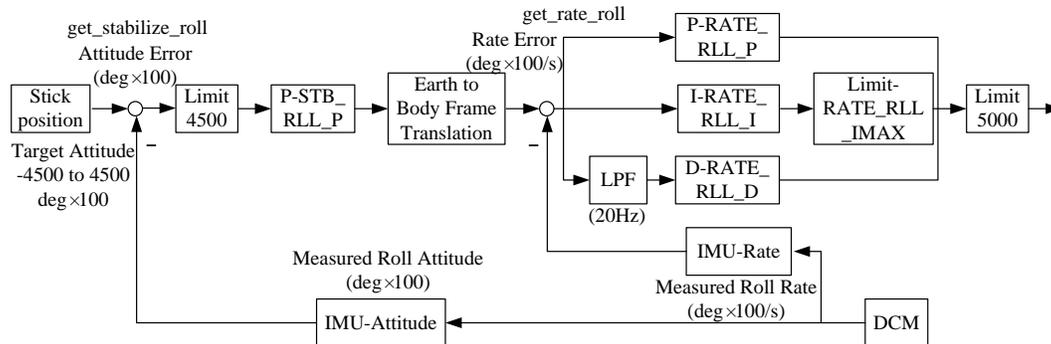
Figure4. Structure diagram of roll controller
