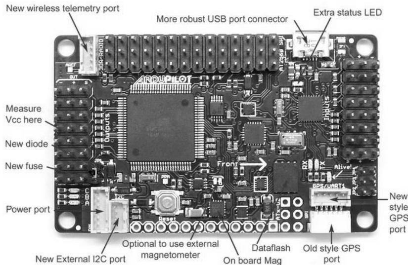
*Figure2. Flight control board*
