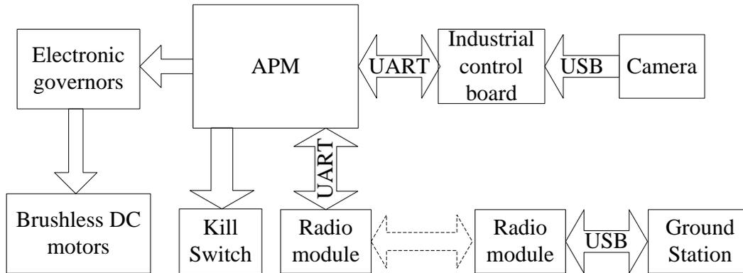
Figure1. Hardware structure diagram of unmanned quadrotor helicopter
