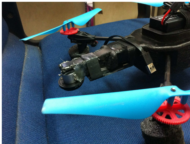
Figure 5. The frontal camera is configured to face down
