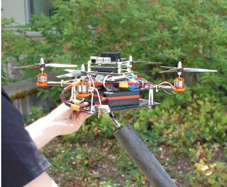
*Figure 9: Quadrotor on test mount.*
