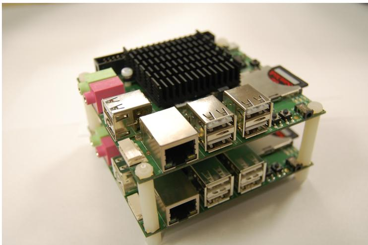
*Figure 6: Stack of two Odroids.*
