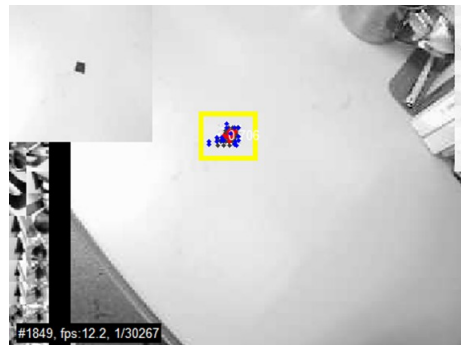
Figure 5: Using the TLD Method to Track a Chip
