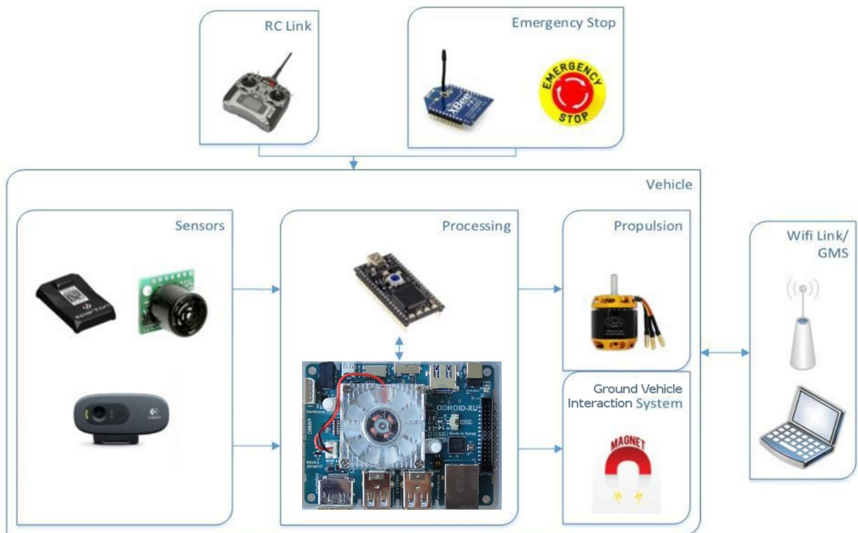
**Figure 1: ERAU RAVEN II System Architecture**
