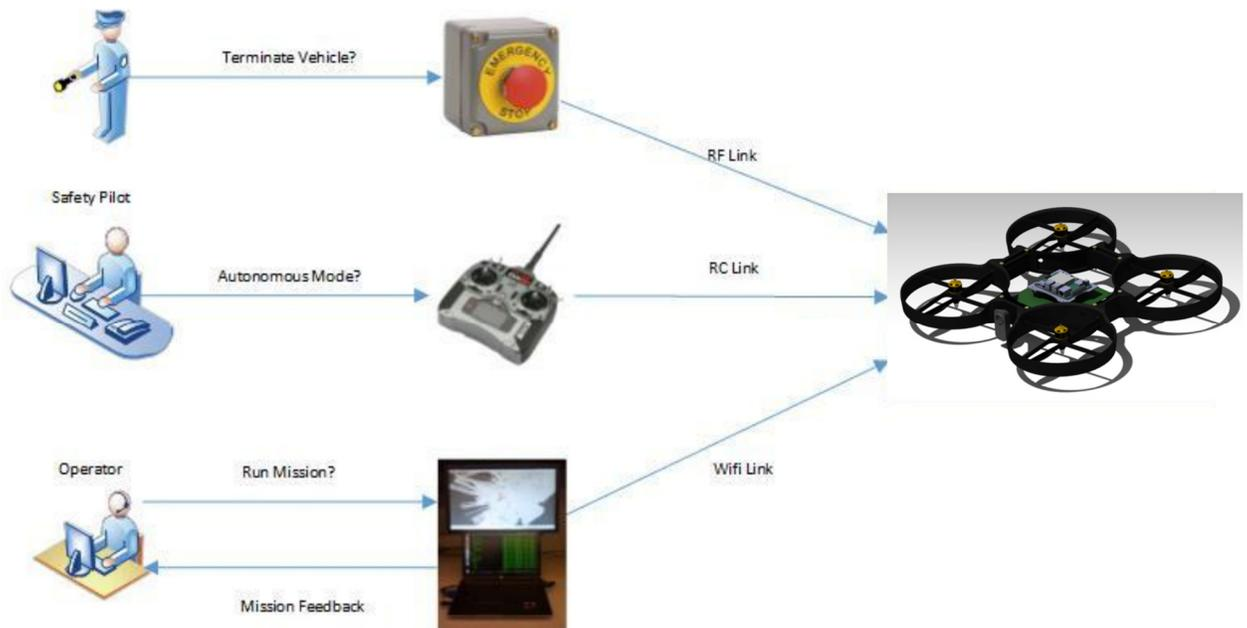
**Figure 4: Man/Machine Interface Hierarchy**
