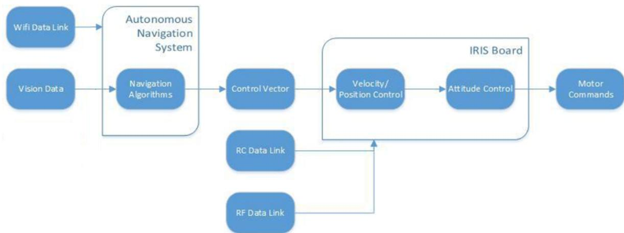
**Figure 3: Control System Architecture**
