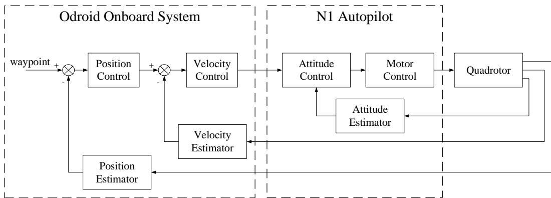
Figure 3. Control system architecture
