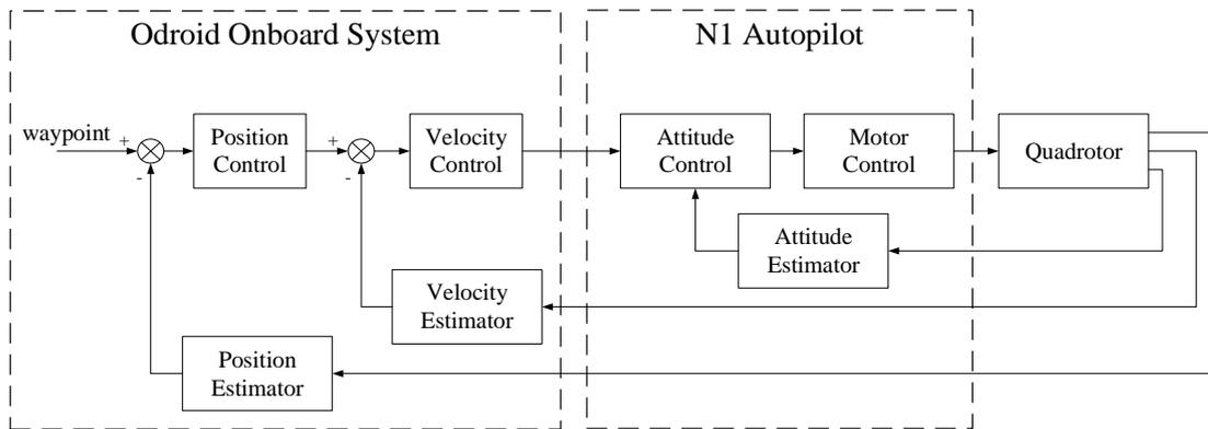
Figure 3. Control system architecture
