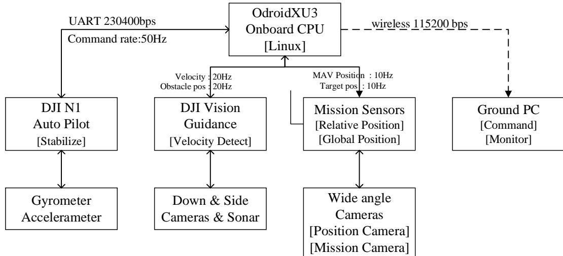
Figure 1. The overall system architecture
