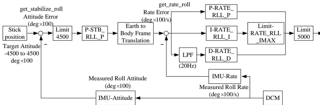
Figure4. Structure diagram of roll controller
