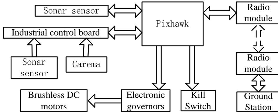
Figure1. Hardware structure diagram of unmanned quadrotor helicopter
