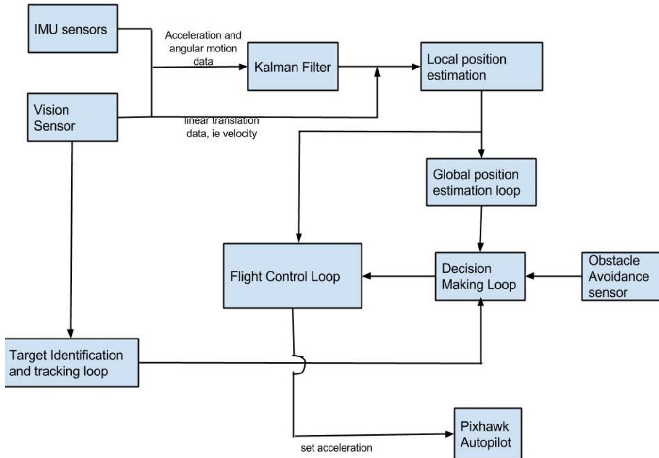
The diagram below shows the flight control system
