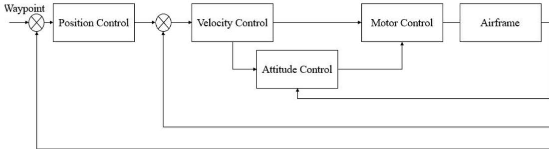
Figure 2: Structure of Control System
