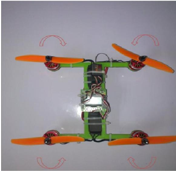
(a) Quad rotor Propulsion and lift system
