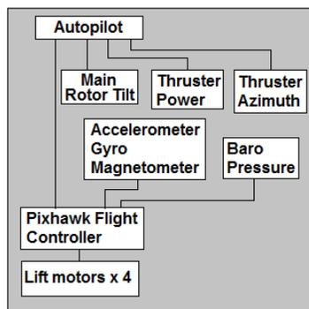
Figure 3. Control system architecture.
