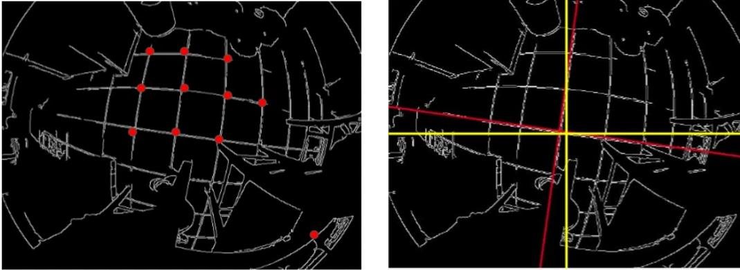
*Figure 8. Grid detection using corner detection (left) and Hough transforms (right)*
