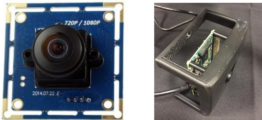
*Figure 6. ELP camera at left. At right is the camera mounted in 3D printed cage with Raspberry Pi computer*
