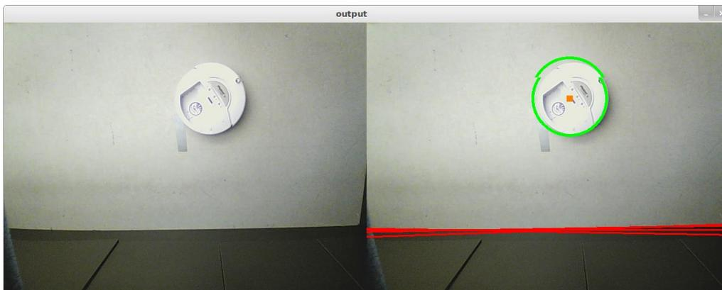
*Figure 4: Example frame from vision processing. This shows proper ground robot detection as well as edge detection.*
