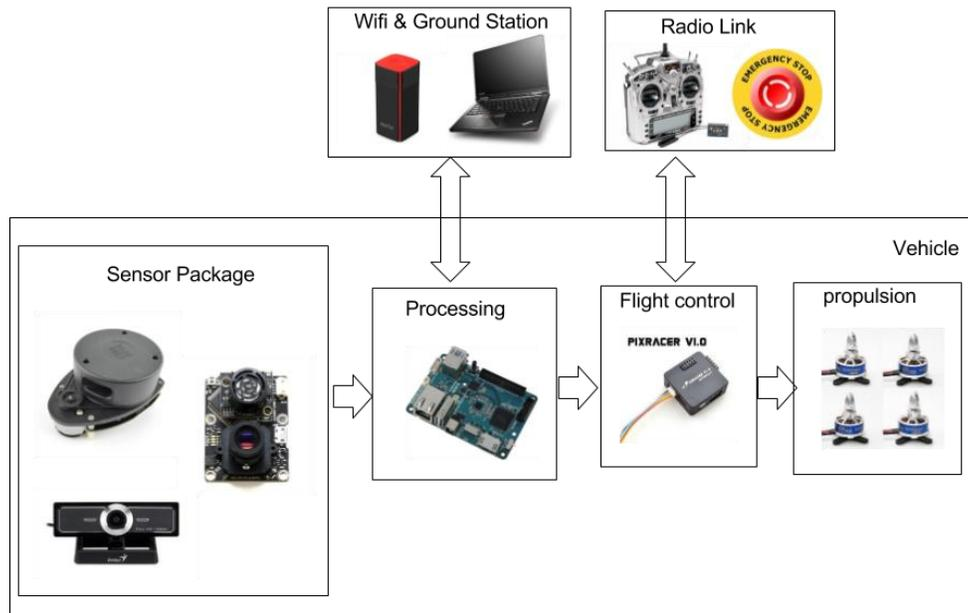
Figure 2. System Architecture
