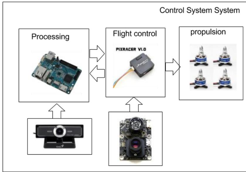
*Figure 3. Control System Architecture*
