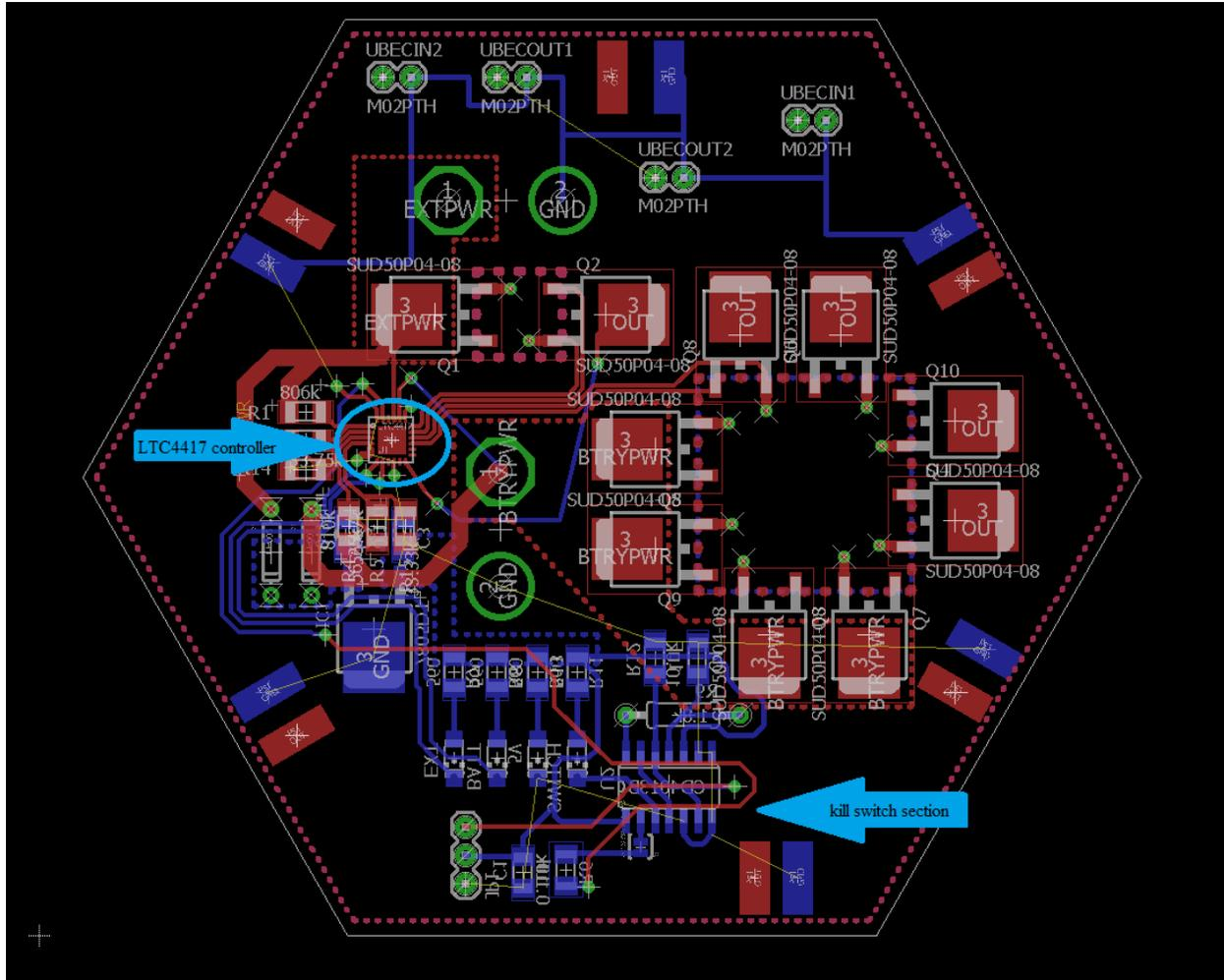
Figure 2: Power Distribution Board
