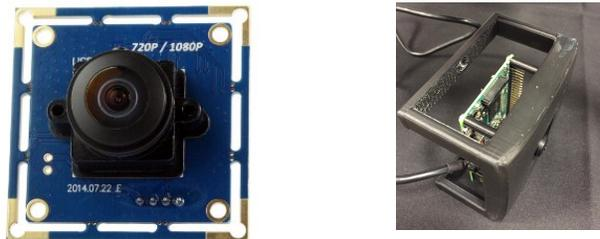
*Figure 5. ELP camera at left. At right is the camera mounted in 3D printed cage with Raspberry Pi computer*
