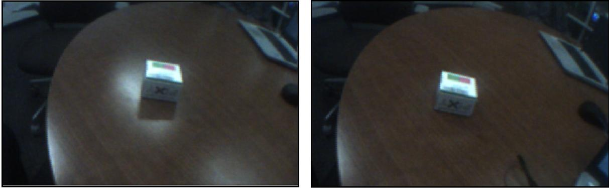
*Figure 6. Glare reduction comparison: without polarizer vs with*
