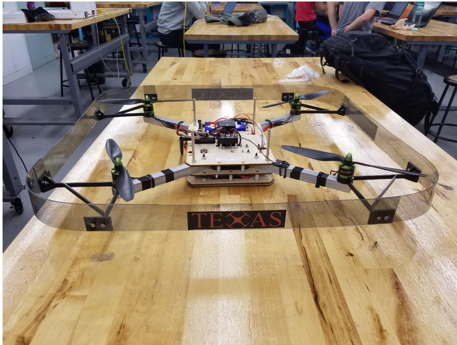
Quadcopter during testing phase
