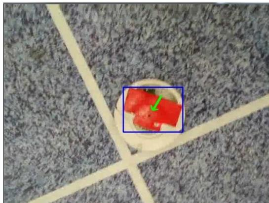
Figure 18. Detecting the movement direction of the ground robot
