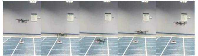
Fig. 17: Snap shots of the UAV during the aerial touch process.
