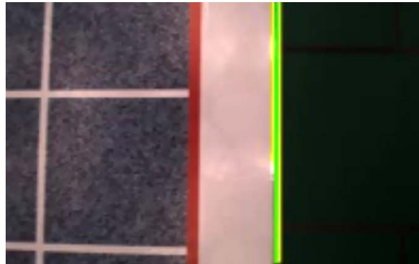
Figure 11: Boundary detection from down-sight camera (boundary is labeled by green line)
